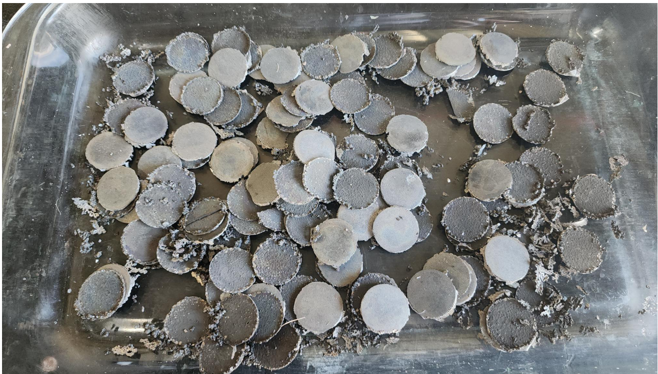
Figure 2 – Cobalt Metal Rounds produced at Cobalt Blue's Broken Hill Technology Centre. Source: Cobalt Blue Holdings.
