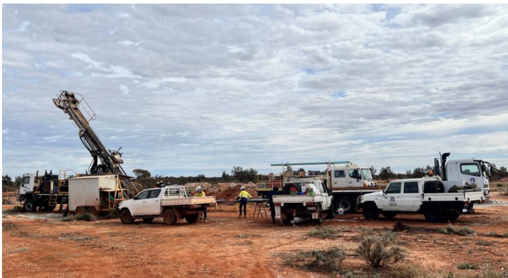
FIGURE 1: DIAMOND DRILLING AT WALLBROOK GOLD PROJECT
