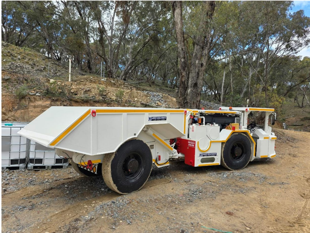
Figure 8 – Bird Systems 10-tonne underground truck ready to commence underground operations at the Reward Gold Mine
