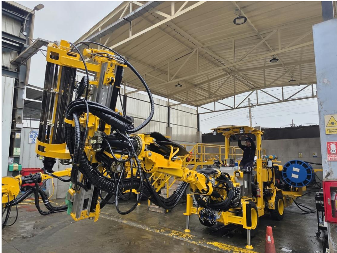
Figure 10 – Vertex Minerals’ Muki LHBP-2R long hole drill at the Resemin factory in September 2026, showing the boom equipped with a magazine
