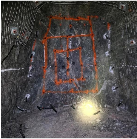
Figure 2 – New smaller drive profile on the Mica veins: face marked up for drilling (left) and completed narrow ore drive (right)
