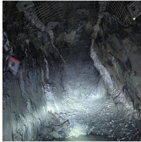
Figure 2 – New smaller drive profile on the Mica veins: face marked up for drilling (left) and completed narrow ore drive (right)
