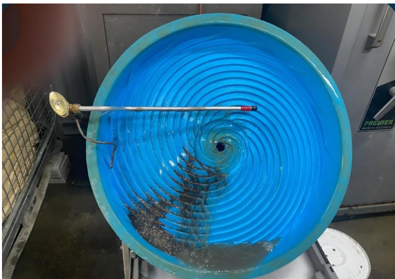
Figure 3 – Spiral wheel upgrading the gold table concentrate (left) and the first gold bar poured at the Reward Gold Mine (right)
