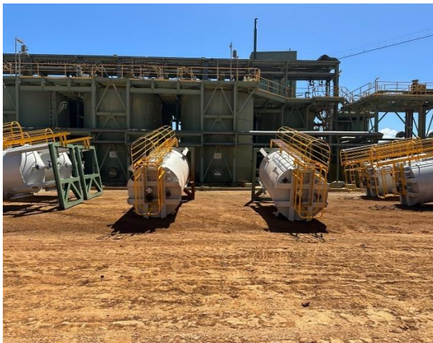
Figure 5: Carbon-in-column tanks installed at Cosmic Boy.
