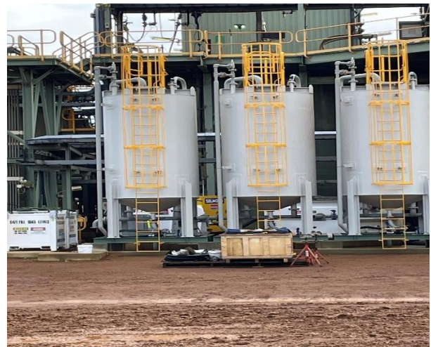
Figure 5: Carbon-in-column tanks installed at Cosmic Boy.
