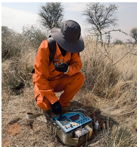
Figure 4. IP fieldwork at Avondschaduw: field personnel and survey equipment (left), and receiver operation (right).
