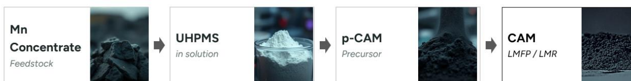
Figure 1. Firebird's proprietary and integrated lithium manganese rich (LMFP & LMR) cathode process commences with the production of ultra-high-purity manganese sulphate (UHPMS).
