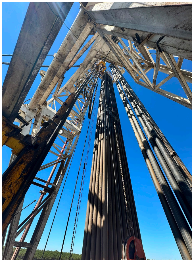
Figure 5: Upward view of the drilling rig derrick and vertically racked drill pipe at Zydeco-1.
