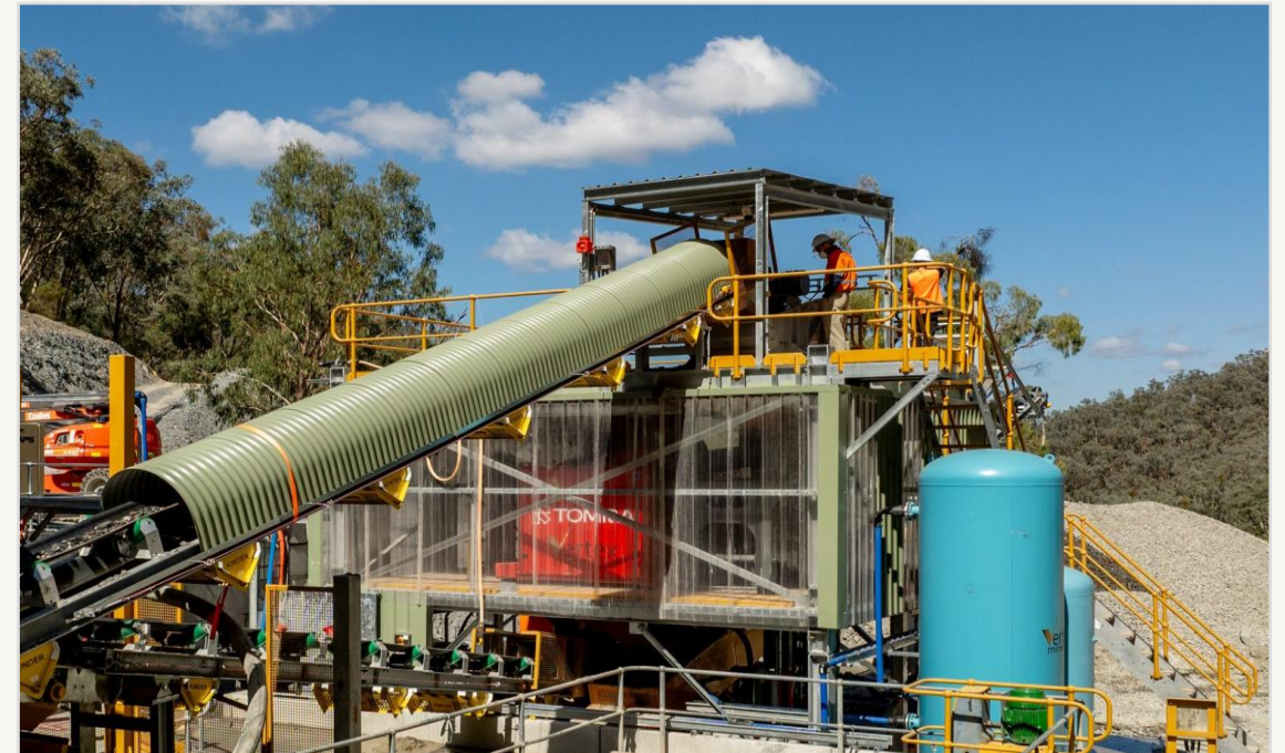
TOMRA ore sorter — laser sorting ahead of the mill.
