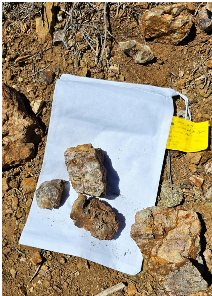
Figure 3 (left): sample WS007, silver-dominant quartz-rich spoil from the pit at the southern end of the central corridor (394 g/t Ag ). Figure 4 (right): sample WS008, silver-rich spoil at the northern end (665 g/t Ag). The two samples presented in Figures 3 and 4 bookend the ~600 m strike of the corridor.
