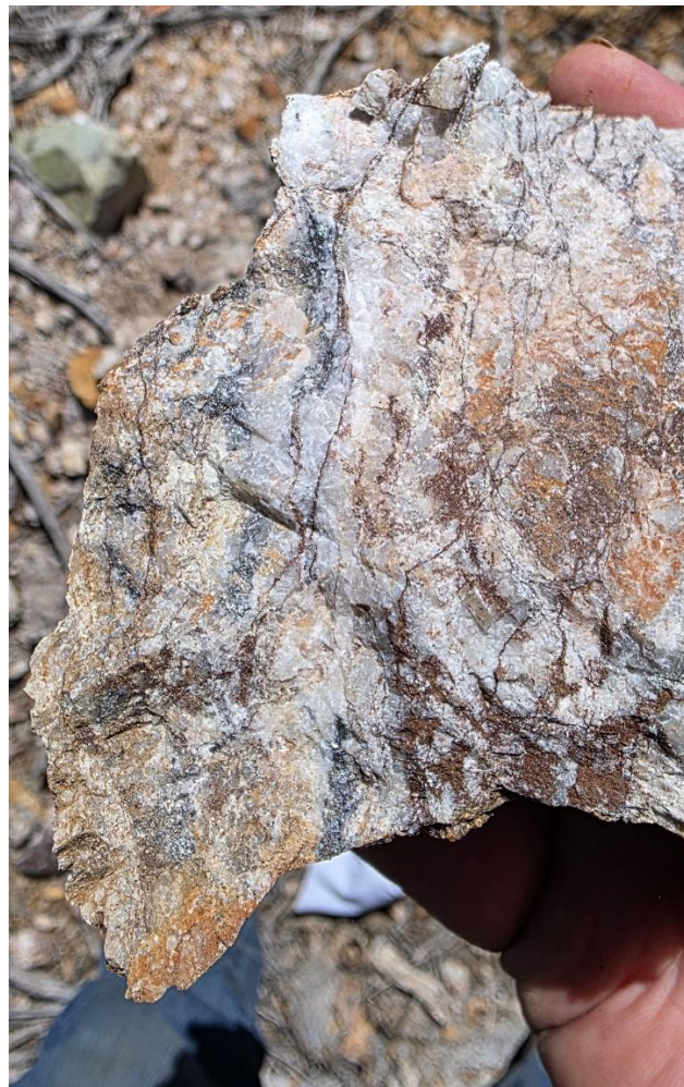
Figure 3 (left): sample WS007, silver-dominant quartz-rich spoil from the pit at the southern end of the central corridor (394 g/t Ag ). Figure 4 (right): sample WS008, silver-rich spoil at the northern end (665 g/t Ag). The two samples presented in Figures 3 and 4 bookend the ~600 m strike of the corridor.
