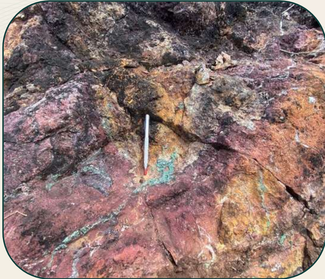
Sample ESR006491 1,2 grading 33.22% Cu Weathered altered ultramafic rock showing quartz stockwork and malachite
