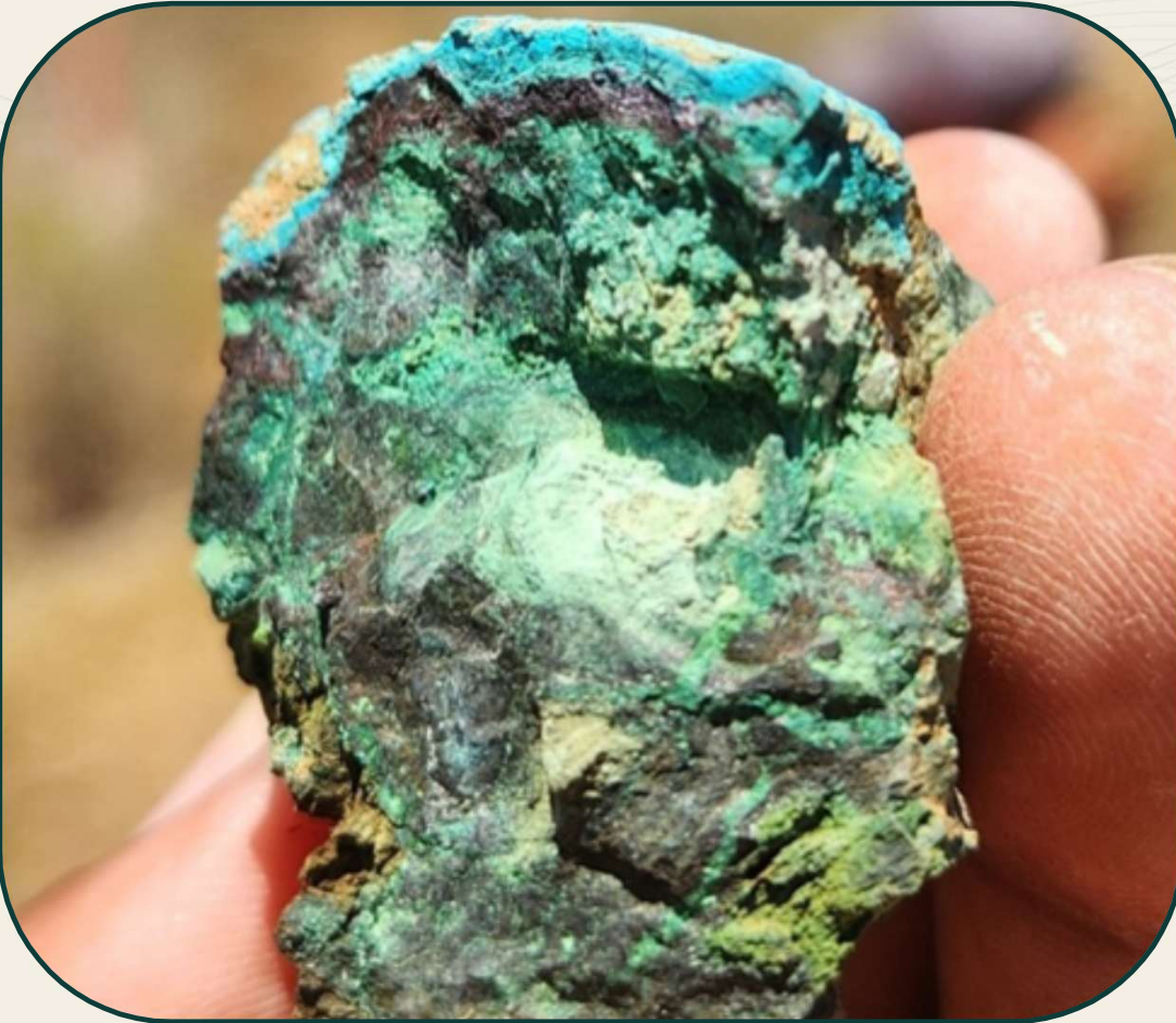
Sample ESR006497 1,2 : Chrysocolla is surface skin (1-2%) overlying an interior of bright green malachite (30-40%), brown goethite (40-50%), along with an unknown yellow-green mineral (~5%) and grey silica (5-10%).
