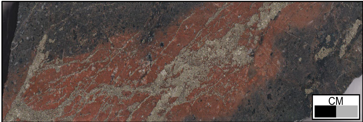
Figure 10: SPD047W1 at 561.4 m, 1 m @ 4.87 g/t Au. Intense potassic selvage surrounding pyrite vein breccia in potassic altered andesite.
