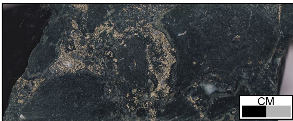
Figure 8: SPD089 at 774.5 m, 1 m @ 6.77 g/t Au. Bladed pyrite-quartz-chlorite breccia fill in chlorite altered basaltic andesite.
