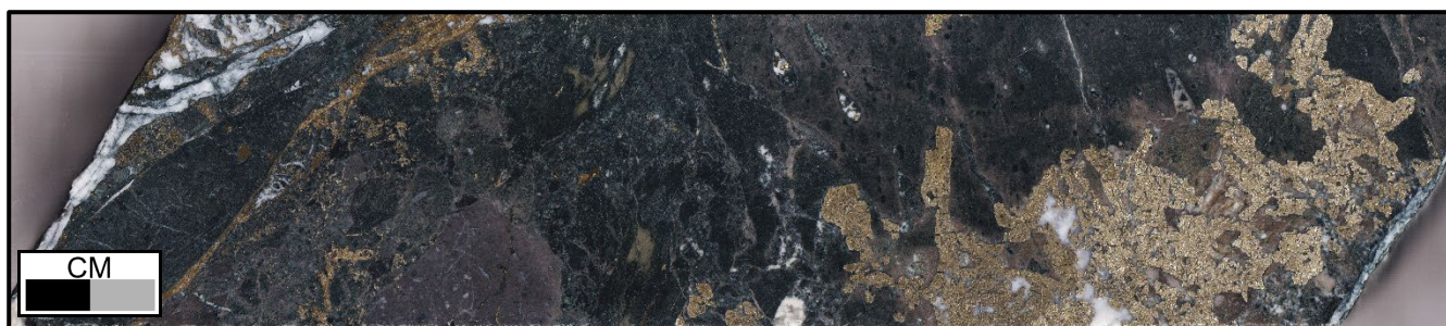
Figure 7: SPD089 at 771.1 m, 1 m @ 4.04 g/t Au. Quartz- pyrite hydrothermal breccia in chlorite- albite altered basaltic andesite.
