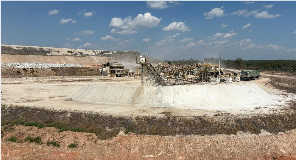
Figure 2 Crusher ore stockpile with ROM pad in the background
