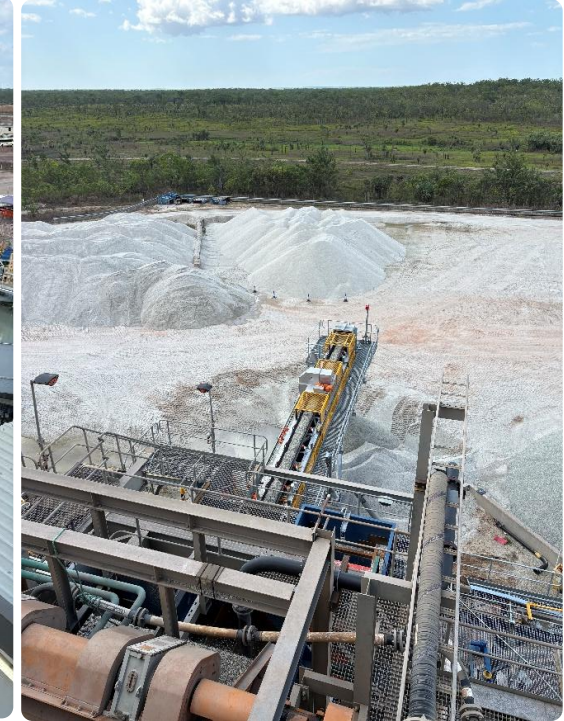
DMS plant brownfields modifications (Left to right) 1. Upgraded rolls crusher screen. 2. Reflux classifier pad. 3. New middlings conveyor
