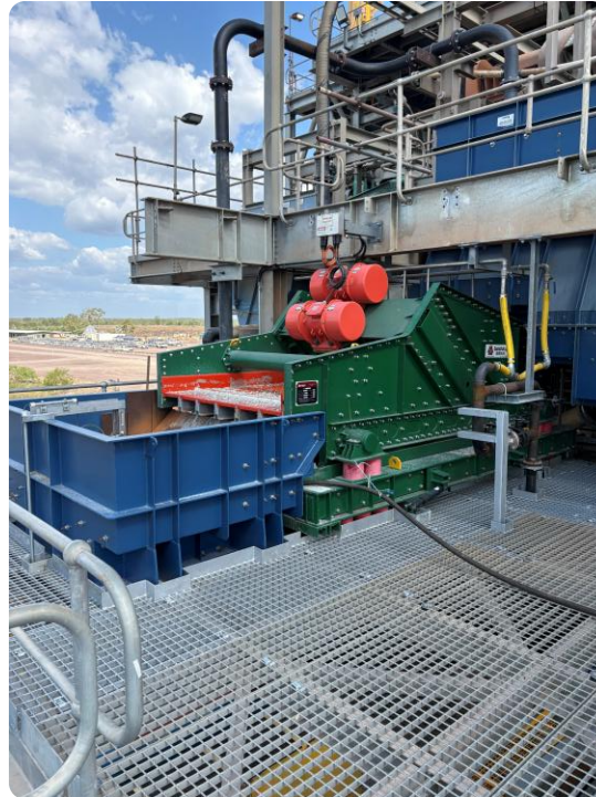
DMS plant brownfields modifications (Left to right) 1. Upgraded rolls crusher screen. 2. Reflux classifier pad. 3. New middlings conveyor
