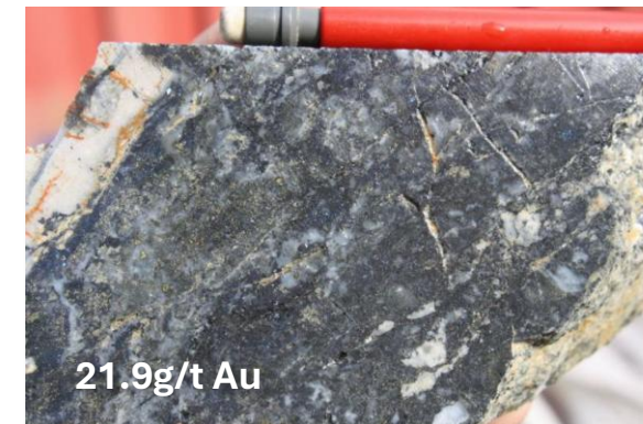
Quartz-polymetallic Au-Ag lode from the Strauss pit area. DDH SRD1, 30.1m, 21.9g/t Au.
