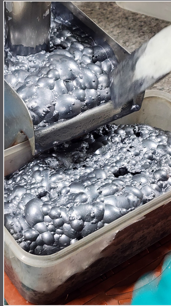
Flotation Testwork on Maronan Silver Lead samples being conducted at AMML Lab in Gosford
