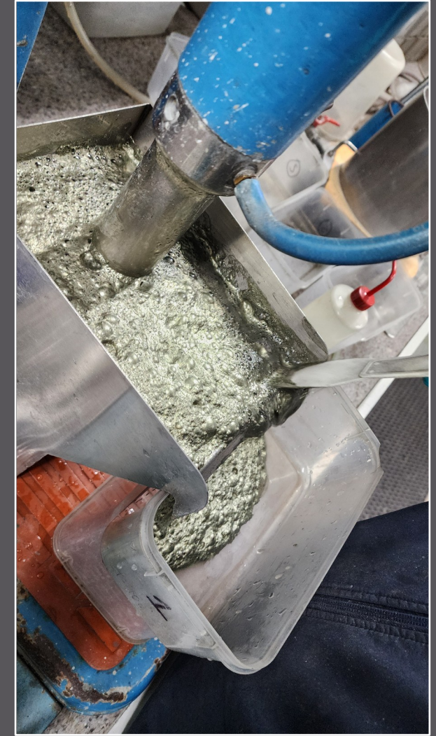
Flotation Testwork on Maronan Copper-Gold samples being conducted at AMML Lab in Gosford
