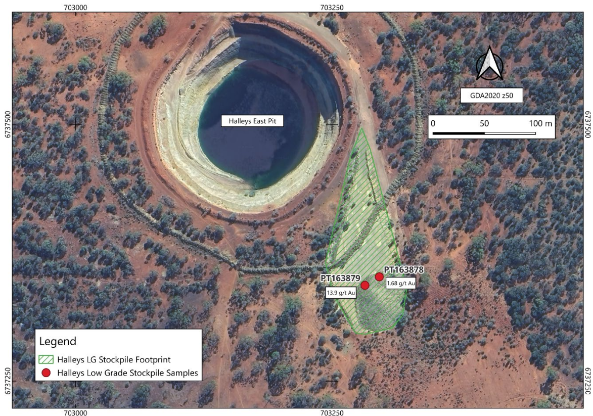
Figure 2. Halley's East pit and low-grade stockpile grab sample locations (GDA2020 / MGA Zone 50)
