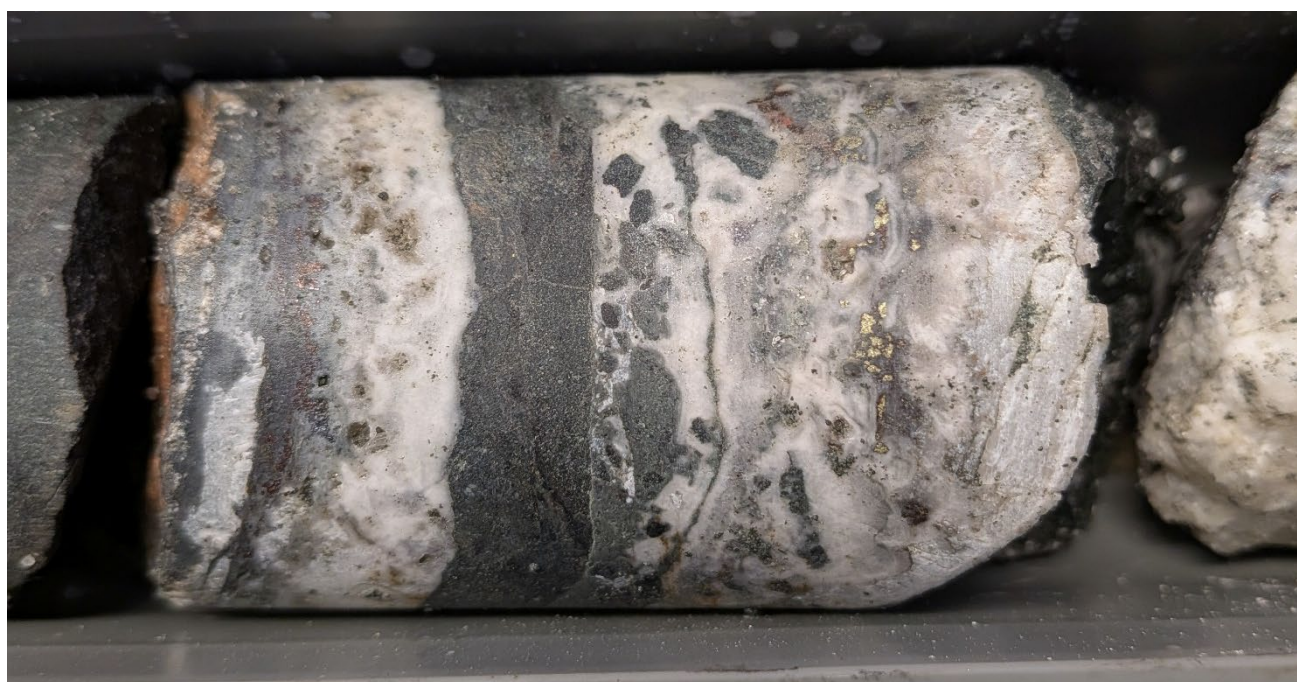
Figure 01 - Photograph of NQ2 diameter drill core from DAN26053. Photograph shows a chalcopyrite-bornite-chalcocite bearing quartz-carbonate vein from logging interval 117-121m downhole.
