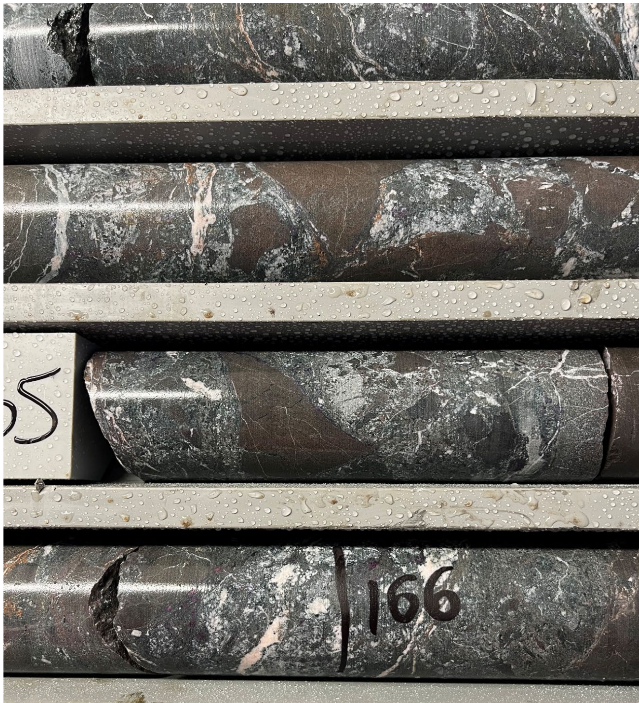
Figure 02 - Photograph of NQ2 diameter core depicting a Danvers-typical chalcocite-bornite bearing breccia from logging interval 160-170.38m downhole, metre mark for 166m observable on the drill core. Drill hole DAN26051.
