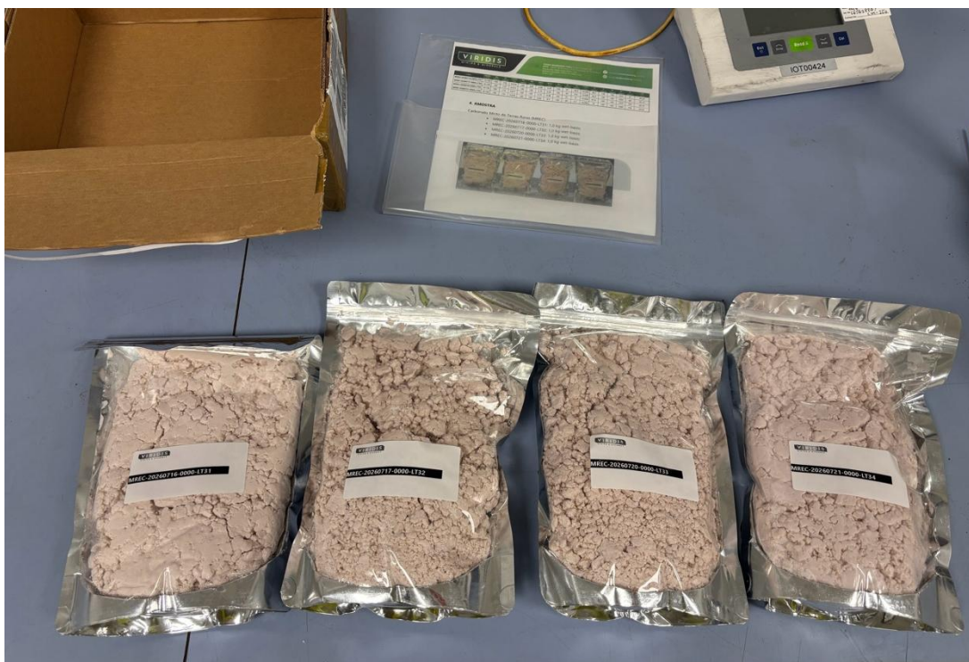
Figure 5: Colossus mixed rare earth carbonate (MREC) samples received in Belfast for initial refinery separation testwork.
