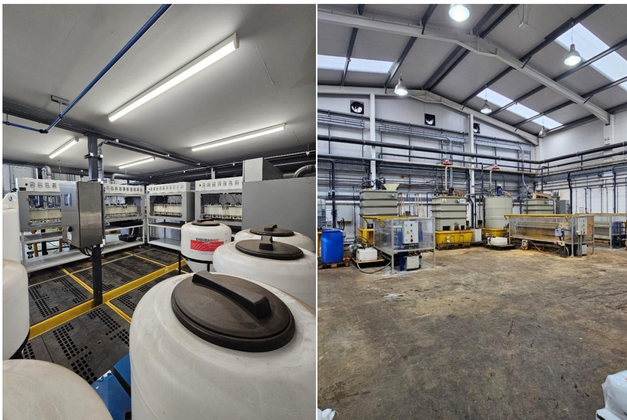
Figure 2: New Heavy Rare Earth Element (HREE) separation circuit (left) and latest Demonstration Plant image including new reactor vessel design and upgraded ventilation system.
