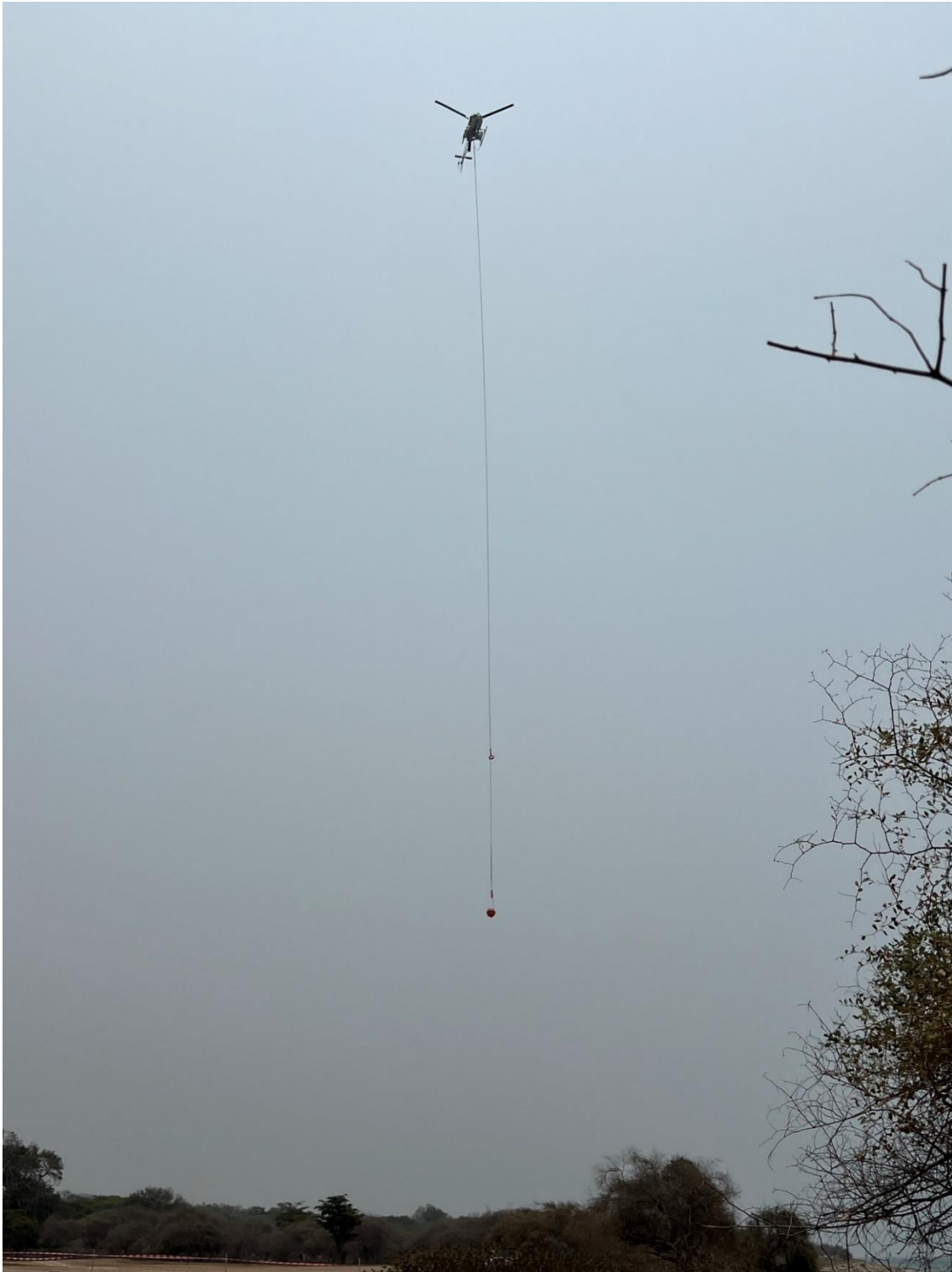
Figure 2: The MT “bird” is the globe at the end of the 90m suspension cord, with the Magnetic Field “bird” 20m above it, suspended beneath the helicopter as the survey commences.
