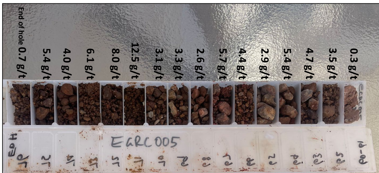
Figure 1: EGR005 drill hole chip tray showing gold assays down hole 15m @ 4.8g/t Au from 61m to end of hole.
