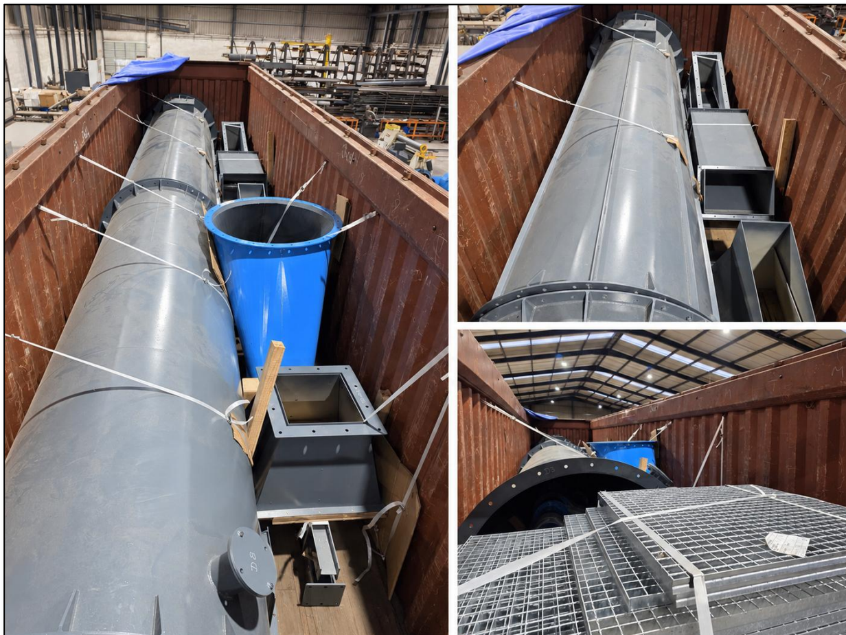
Figure 3 - Chutes, process equipment structures, piping and associated steelwork fabricated at the Arliz facility in Portugal and loaded for shipment to the Cabinda Phosphate Project in Angola.
