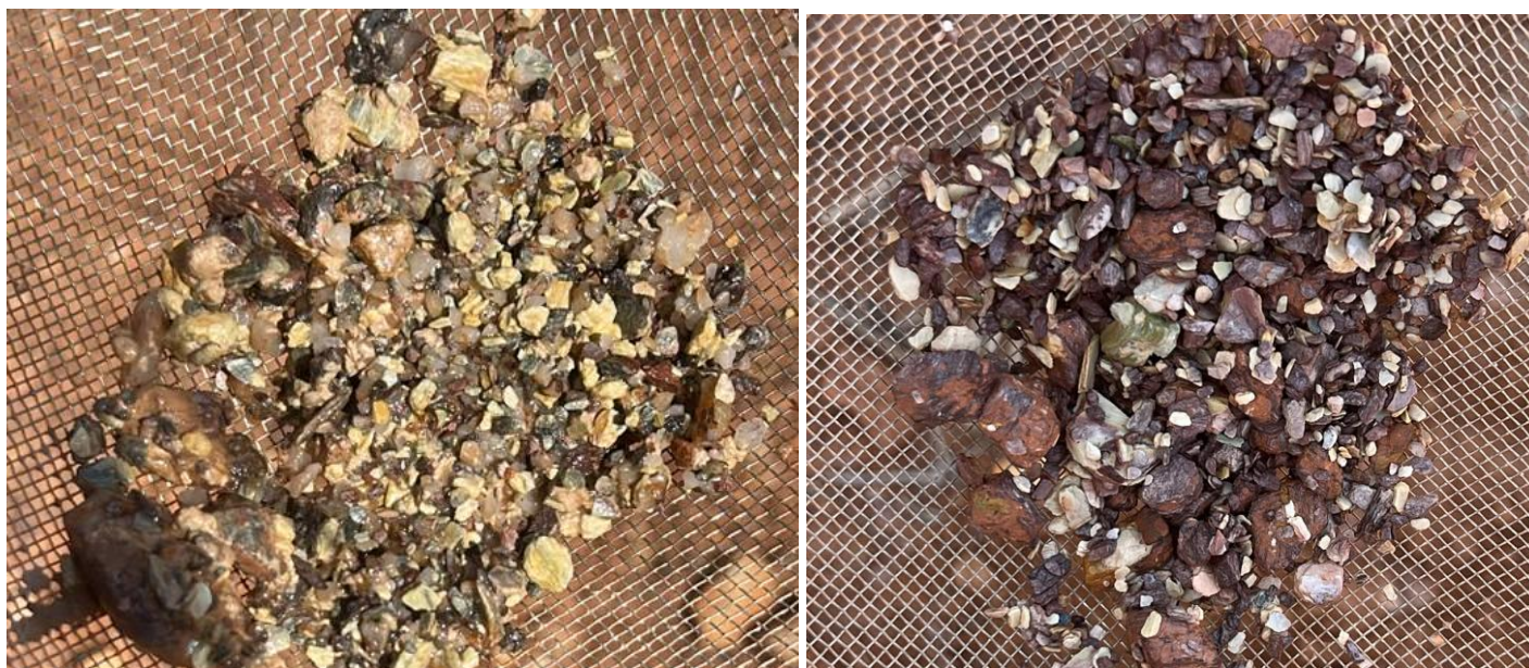
Figure 1: Photographs of mineralised aircore drill cuttings from ABAC008 at German Well South. (Left) Highly weathered and oxidised shear zone containing approximately 30% quartz veining from 63–64 m, returning 10.0 g/t Au . (Right) Strongly iron-oxide-rich, oxidised shear zone (saprock) from 72–73 m (end of hole), returning 0.8 g/t Au .
