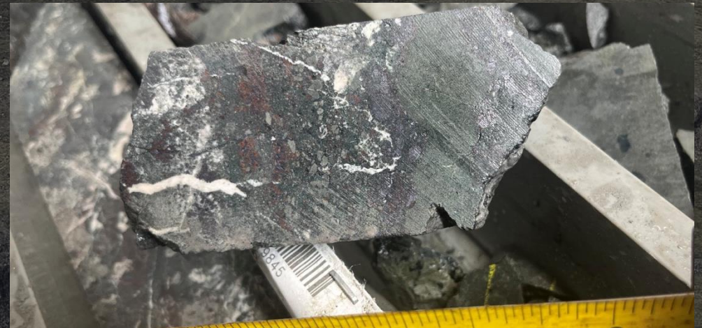
Figure - Photograph of halved NQ2 diameter core showing mixed chalcocite and bornite mineralisation in the chlorite breccia zone at 45.5m in DAN26026
