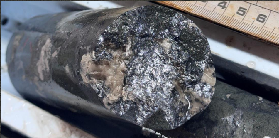
Figure - Photograph of NQ2 diameter core containing coarse grained chalcocite breccia cement from between 175.4-179.3m in downhole in DAN26036. Interval returned 3.90m @ 16.45% Cu and 31g/t Ag from 175.4m
