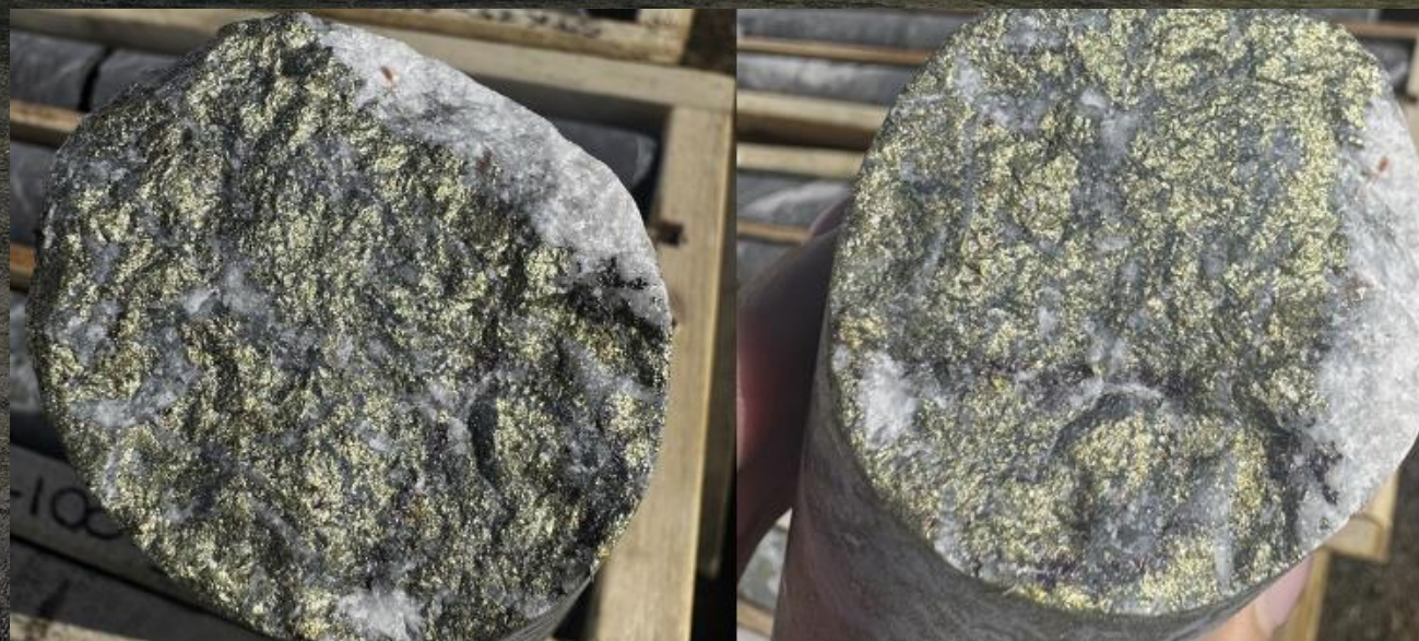
Chalcopyrite-bornite-quartz-carbonate veining below the base of the sedimentary sequence in STK25001 at 291.4m, which assayed 14.95% Cu & 0.51g/t Au. Core diameter is NQ2
