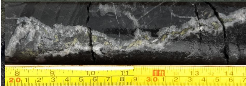
Example of chalcopyrite-bornite hosting quartz-carbonate veining in STK25001 between 181.30 and 181.52m downhole. Core diameter is NQ2.
