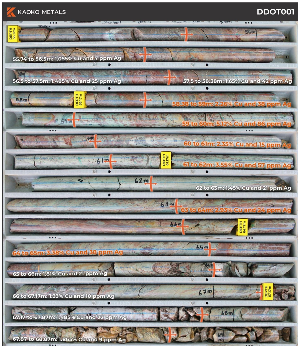
Figure 3 - DDOT001 drill core from 55.74 to 68.87m showing copper mineralisation and associated assay grades (refer to Appendix A for full assay details).
