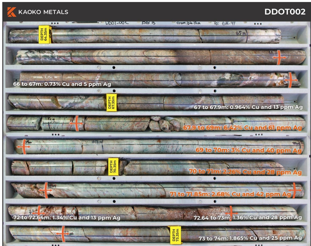
Figure 4 – DDOT002 drill core from 66.00m to 74.00m showing copper mineralisation and associated assay grades (refer to Appendix A for full assay details).
