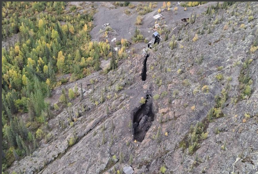
Contact Lake Adit & Collapsed Stope
