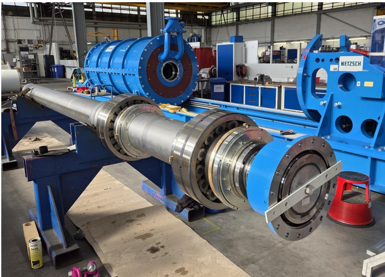
Figure 12 – IsaMill and shaft, preparing for shipment
