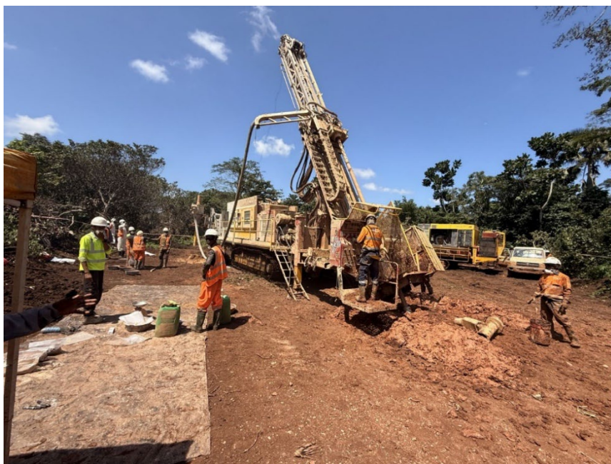
Figure 6. RC rig drilling at the Bondoukou Gold Ridge Project.
