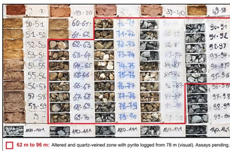
Figure 1a. Drill chip trays from hole BDR010C, 50–100 m (1 m intervals). The red outline marks the altered and quartz-veined zone logged visually from 62 m to 96 m, with pyrite logged from 78 m (78–84 m and 90–96 m); the pyrite occurrence logged for each interval is set out in Table 1. Assays are pending.
