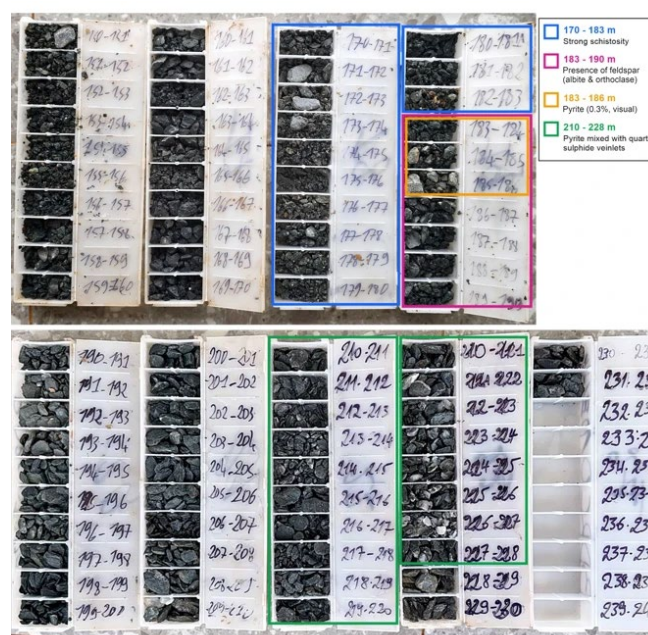
Figure 1b. Drill chips from hole BDR010C, 150–232 m, showing strong schistosity (170–183 m), feldspar with pyrite (183–190 m) and pyrite with quartz–sulphide veinlets (210–228 m). Refer to the cautionary statement on visual estimates on page 1.
