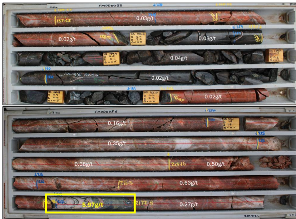
Figure 6 Core photos from FMDD0058 with gold grades (white): top, 157.52–161.36 m, unaltered lamprophyre (158.8–161.0 m); bottom, 213.3–217.73 m, silica-carbonate altered and sheared quartz syenite intruded by lamprophyre (216.96–217.20 m), bounded by high-grade quartz veins (yellow box see below Figure 6) (ICL ASX 29 September 2026)
