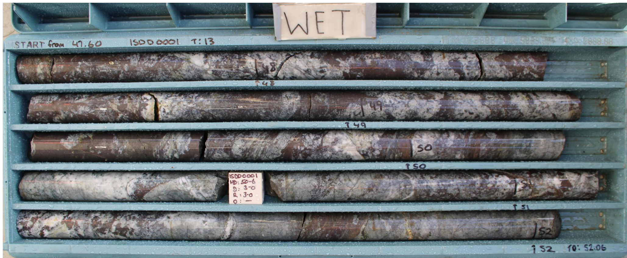
Figure 5 ISDD001 – Zone of sphalerite dominant sulphide mineralisation with lesser amounts of pyrite, galena, pyrrhotite and chalcopyrite hosted by quartzite breccia.
