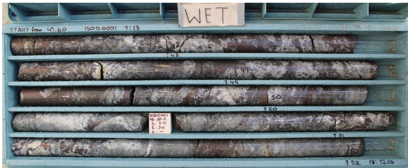
Figure 1 ISDD001 – Zone of sphalerite dominant (brown) sulphide mineralisation hosted in a quartzite breccia
