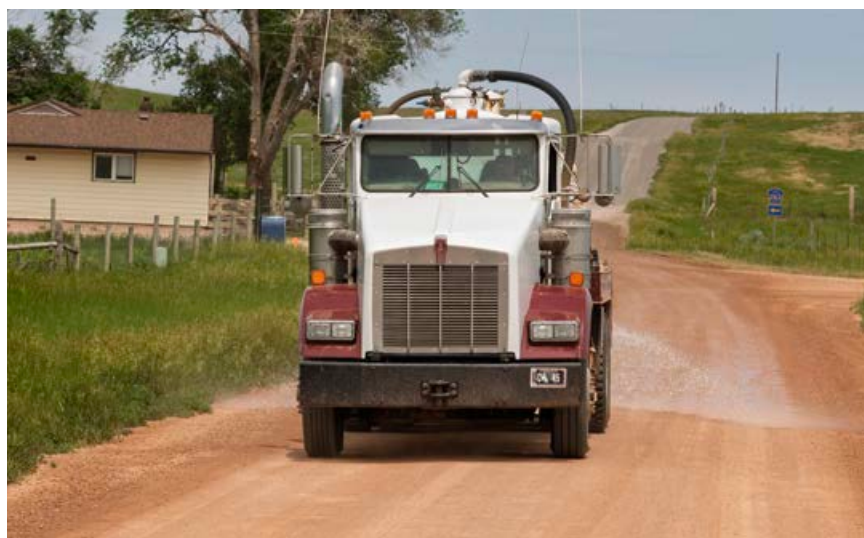
Figure 4-3: Water tanker performing dust control
