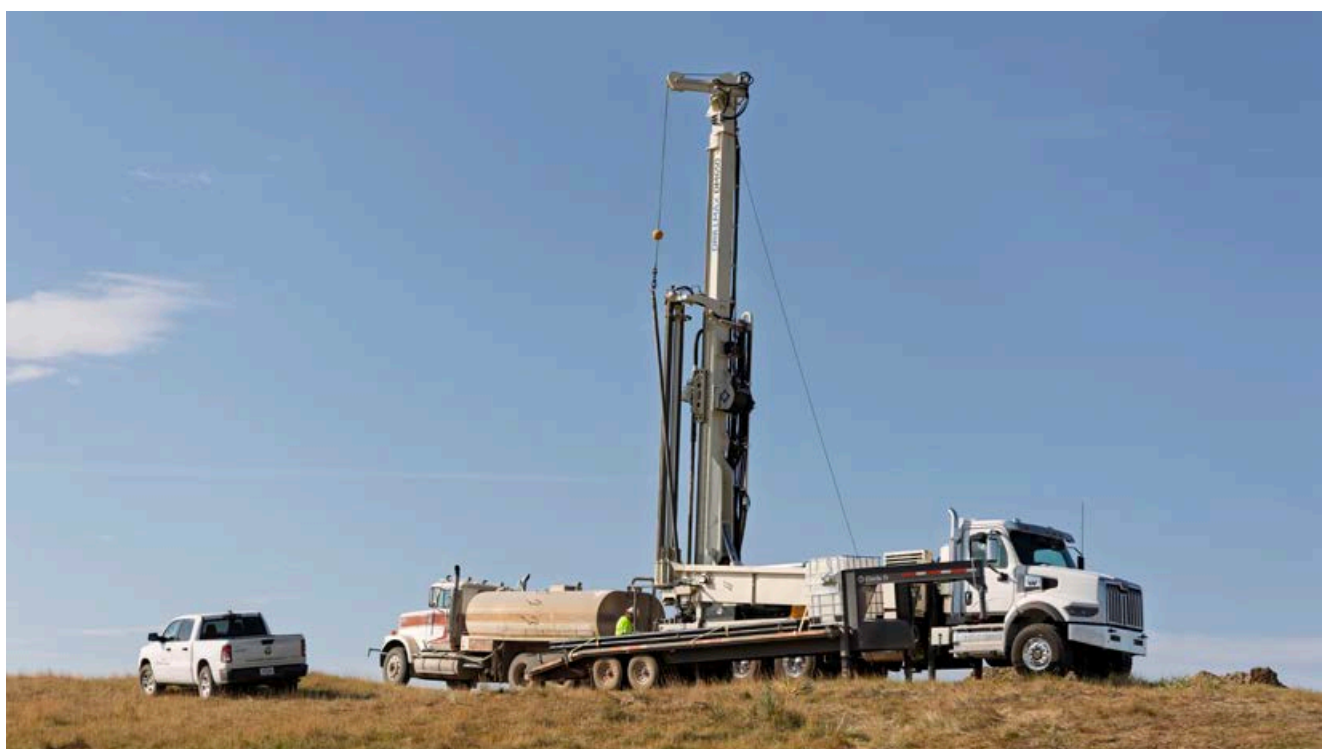
Figure 4-7: Strata's in-house drill rig conducting delineation drilling at Mine Unit 5
