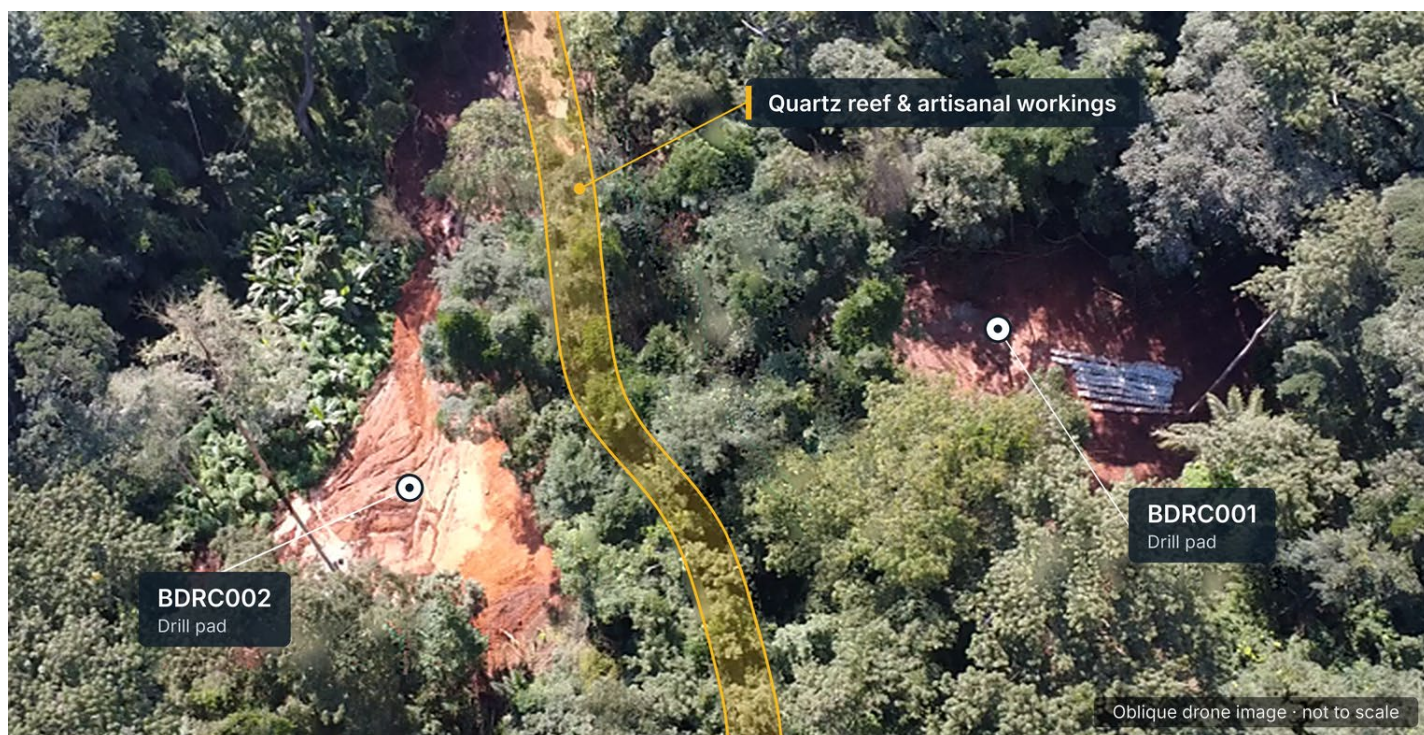
Figure 2. Oblique drone image of the Wilfred target at Bondoukou Gold Ridge, showing the BDRC001 and BDRC002 drill pads either side of a quartz reef with artisanal workings. The two holes were drilled as a scissor pair (BDRC001 to 045°, BDRC002 to 225°) to test the reef and its extensions at depth. Not to scale.
