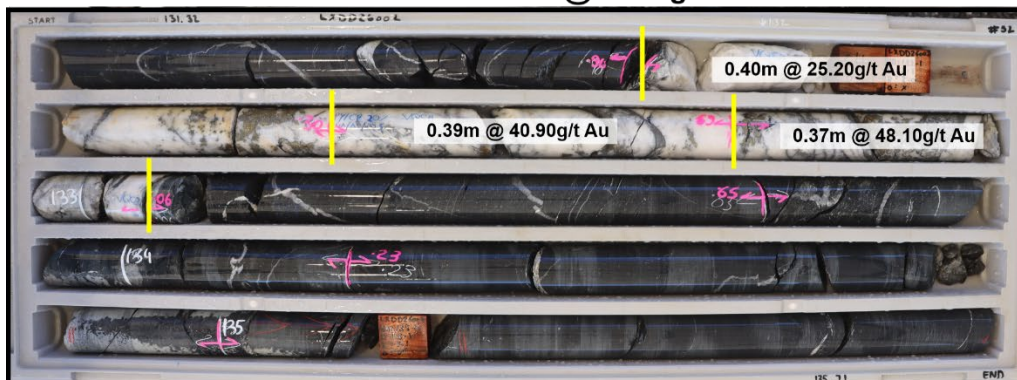
Figure 3: Core photos of recent surface diamond holes LXDD26007(top) and LXDD26002(bottom) showing significant intercepts referenced in the body of this announcement.
