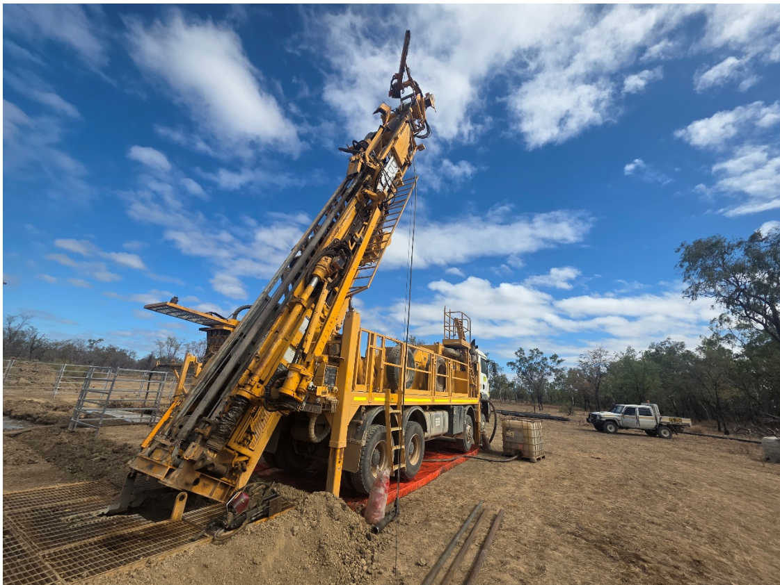
Figure 1 – Diamond drill rig on site at the Bulimba Gold Project
