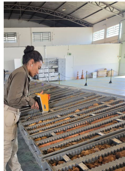
Photos 4-6: Oceana's Senior Geologists Helena (left) and Giovanna (centre and right) undertaking spot checks with a Vanta pXRF to determine zones of diamond core to be sampled for laboratory assay. This follows lithological logging and core tray photography at Oceana's office and core facility in Patrocínio.
