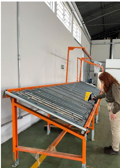
Photos 4-6: Oceana's Senior Geologists Helena (left) and Giovanna (centre and right) undertaking spot checks with a Vanta pXRF to determine zones of diamond core to be sampled for laboratory assay. This follows lithological logging and core tray photography at Oceana's office and core facility in Patrocínio.
