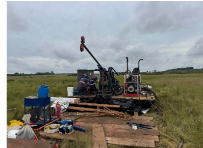
Photos 1-3: Third diamond drill rig is now set-up at the Central REE target area and has started drilling overnight. The man-portable rigs are placed on timber platforms to minimise ground disturbance.
