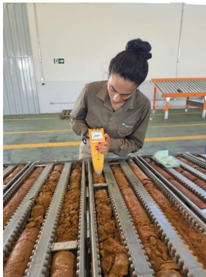
Photos 4-6: Oceana's Senior Geologists Helena (left) and Giovanna (centre and right) undertaking spot checks with a Vanta pXRF to determine zones of diamond core to be sampled for laboratory assay. This follows lithological logging and core tray photography at Oceana's office and core facility in Patrocínio.
