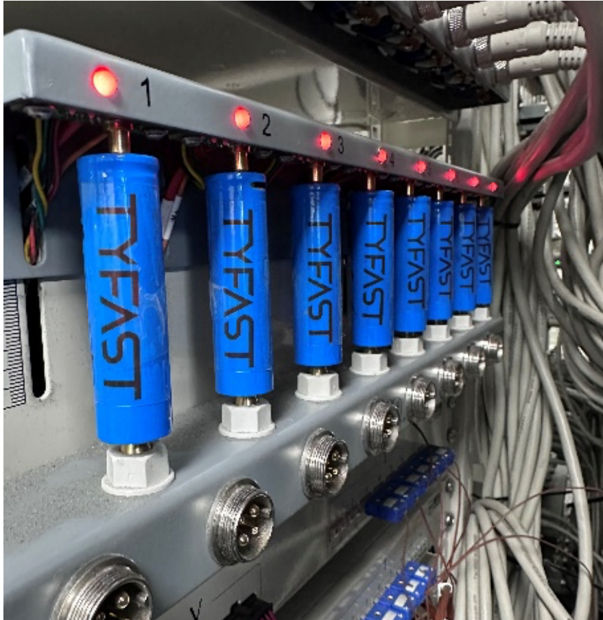
Figure 1: Tyfast cylindrical lithium vanadium oxide LVO cells undergoing cycling
