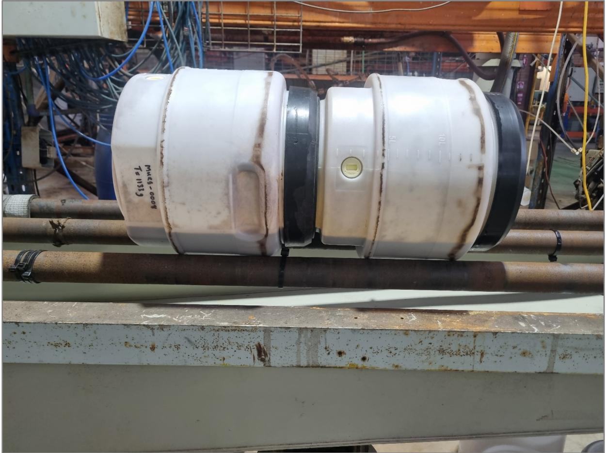
Figure 5: Bottle Roll Test Work set up.
