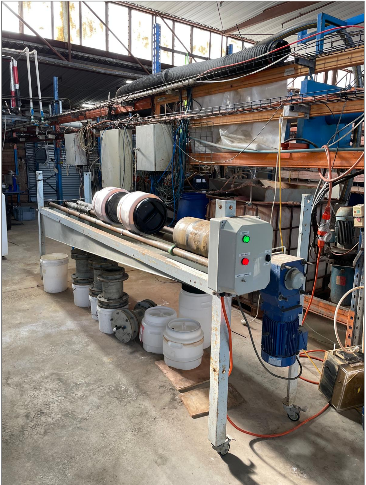
Figure 4: Bottle Roll Test Work set up.
