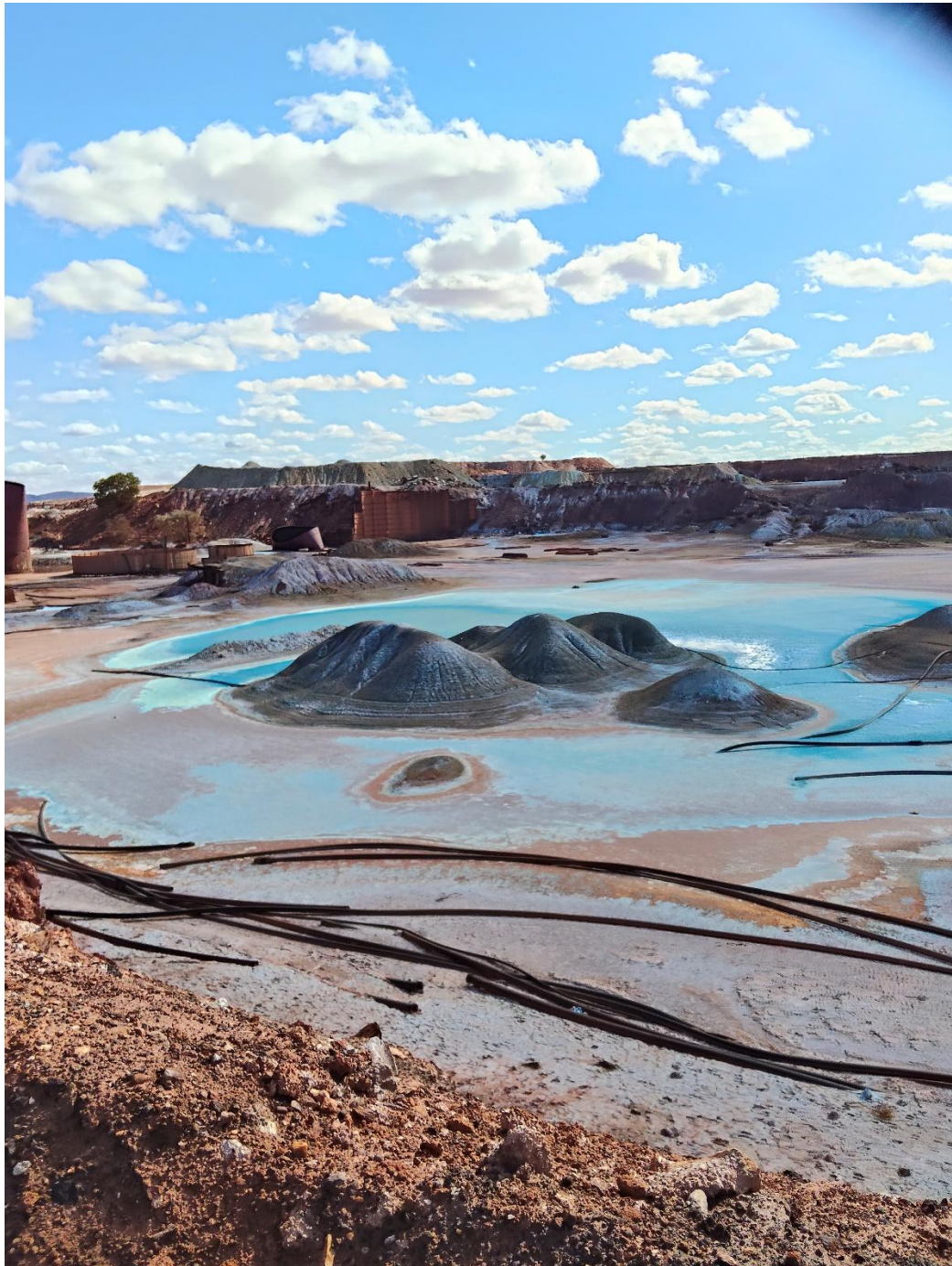
Image 1: Copper oxide and sulphate precipitate material within the former flotation crushed ore stockpile at Horseshoe Lights.
