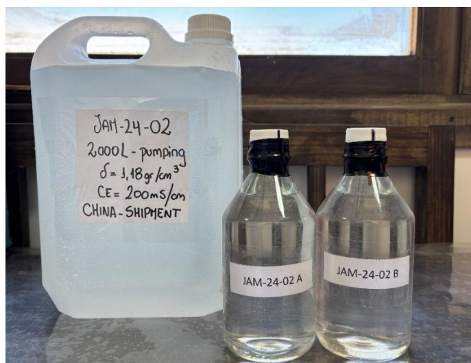
Figure 4. Brine sample shipped to Ekosolve pilot plant for testing. It had a high SG value.
