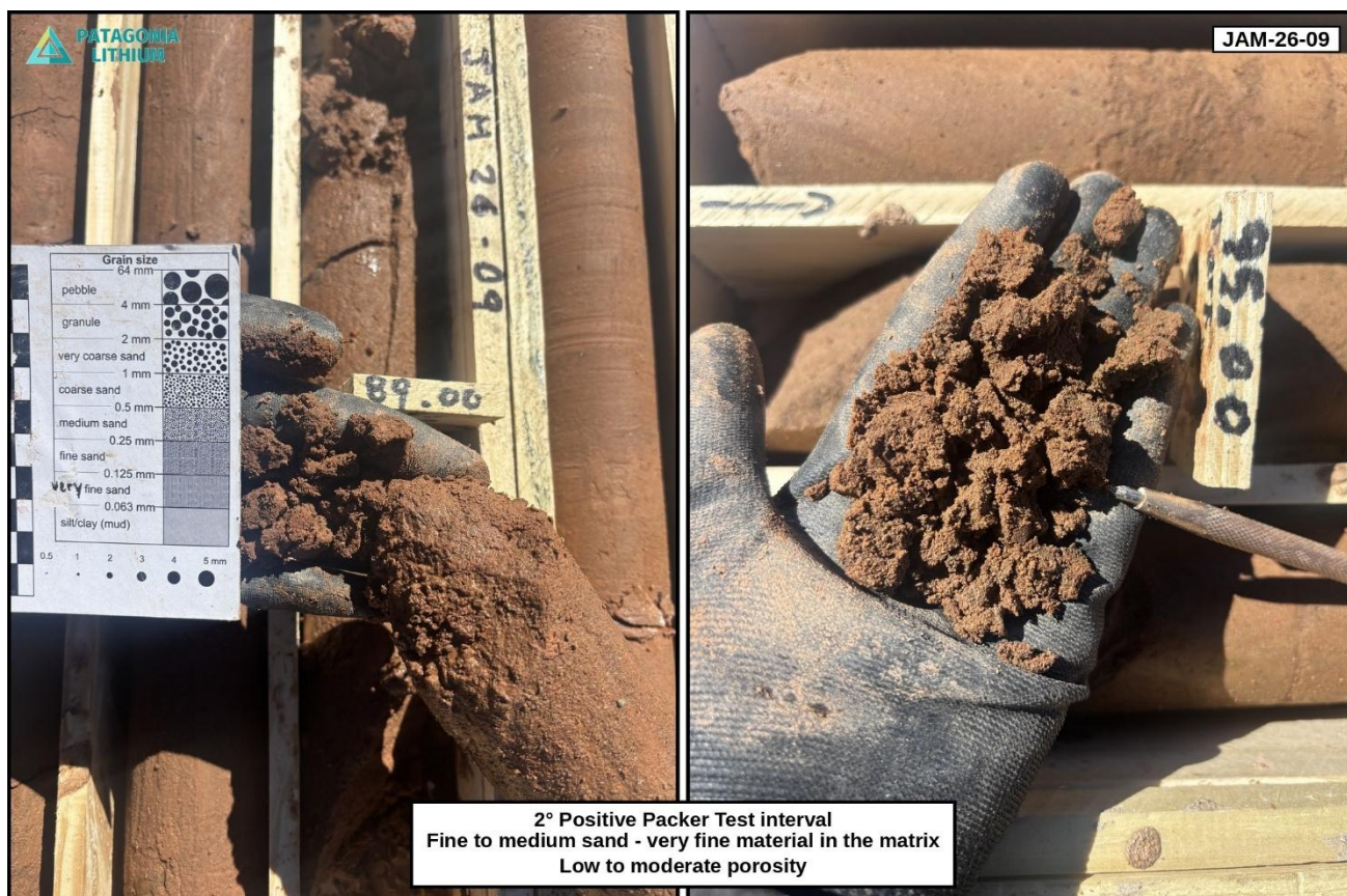
Figure 1. Core at 95m is composed of sandy clays visually with low porosity but still transmitting brines for a successful packer test on 23/9/2026.
