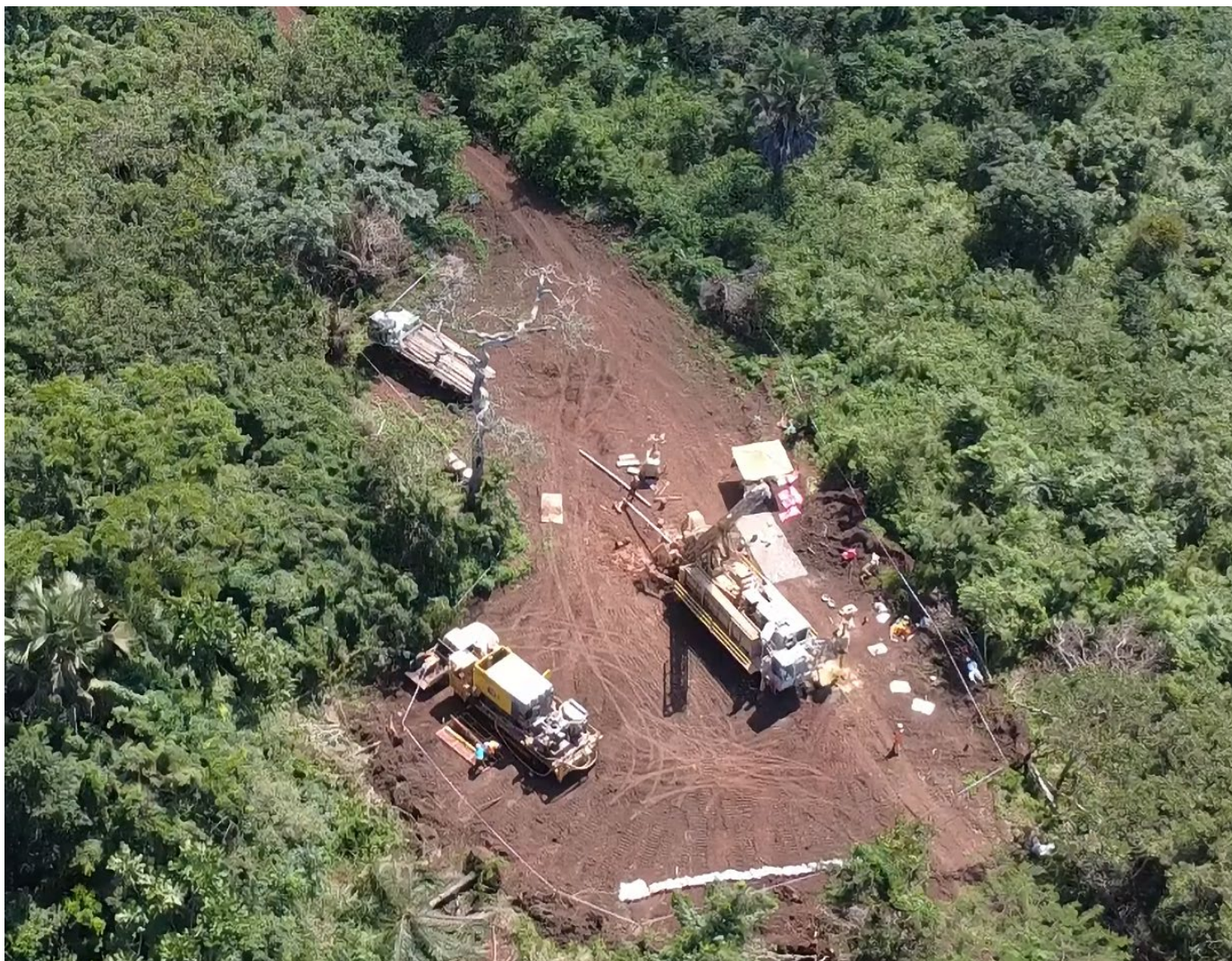
Figure 6. Aerial view of the RC rig on a drill pad at the Wilfred target.
