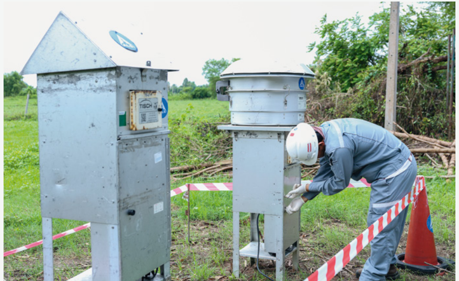
A specialist from ALS, an independent environmental consultant, measures dust and air quality levels at one of the monitoring stations around the Chatree Community.
