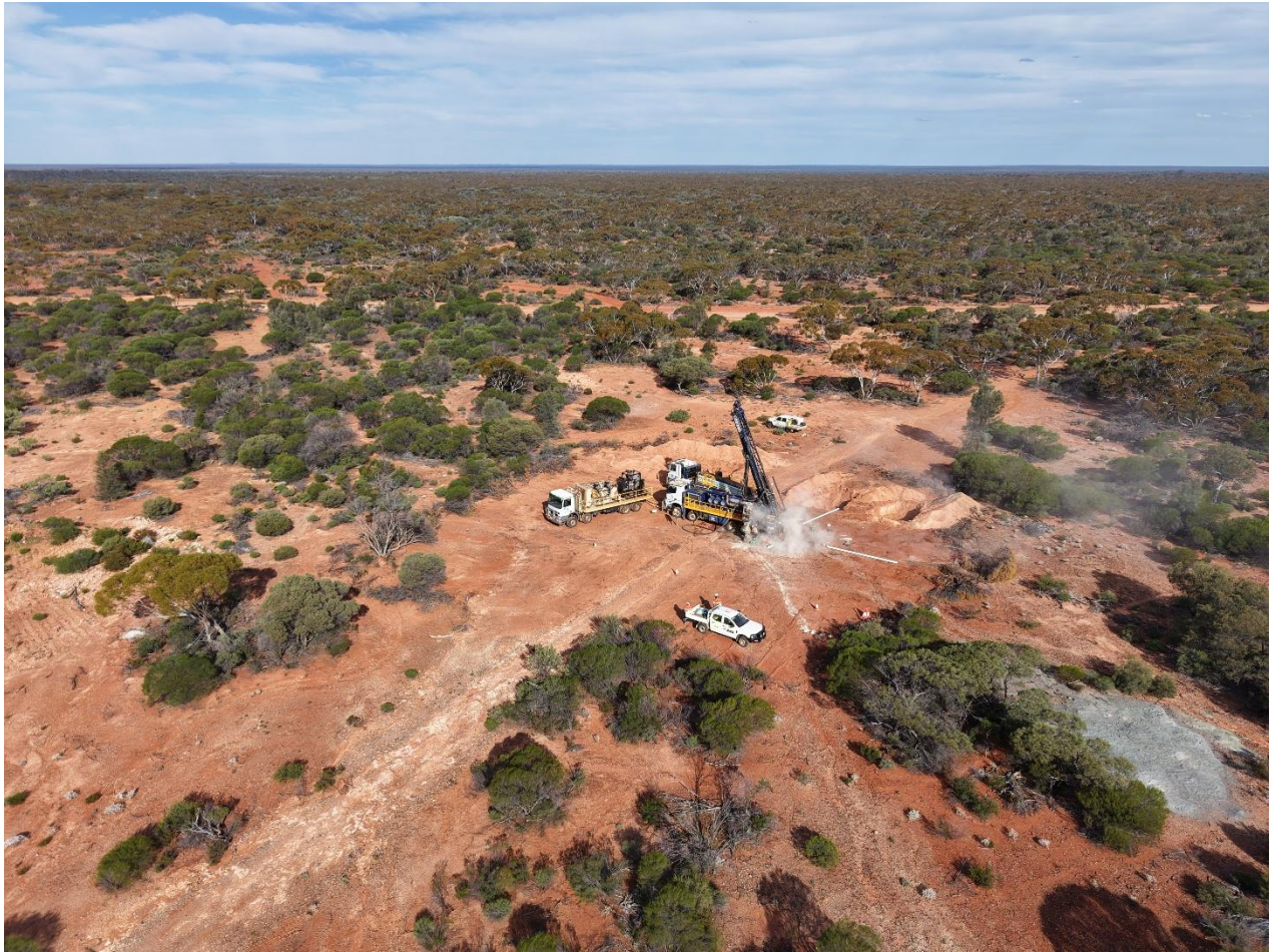
Image 1: RC Drill rig on site at First Hit.
