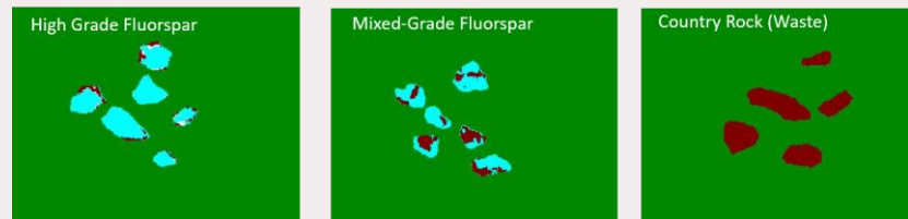
Laser ore-sorting technology by TOMRA applied to Quinn Project metallurgical samples, showing clear differentiation of ore types and waste. Samples approximately 10-15mm
