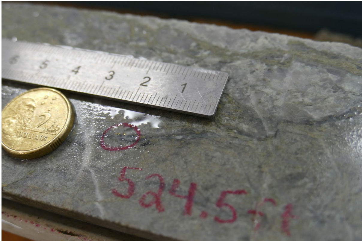
Image 3: 26FRD001 HQ3 core (cut) at approximately 524.5ft (159.9m) downhole showing visible native gold blebs associated with sericite altered brecciated metasediment near boudinaged quartz-carbonate veining and pyrite mineralisation. Scale shown in cm/mm with a 20.5mm diameter coin.
