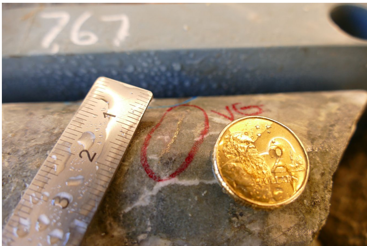
Image 1: 26FRD001 core at approximately 767ft (233.8m) downhole showing visible native gold veinlet extending for more than 1cm; associated with quartz-carbonate veining and pyrite mineralisation. Scale shown in cm/mm with a 20.5mm diameter coin.
