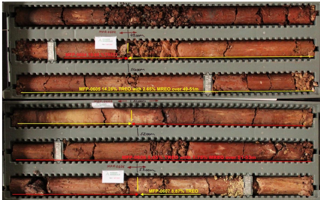
Figure 3. Drill core from MFSR-056 with the intervals marked for high-grade TREO samples MFP-0605 and MFP-0606, and parts of samples MFP-0604 and MFP-0607 (see Table 2). The material is fine-grained, soft reddish-brown, clayey phonolite saprolite. Photograph taken dry before cutting the core. Core recovery was measured at 100% (no core loss) over these intervals. The HQ core shown starts at the top-left, and the downhole direction is to the right; tray rows are one metre long.
