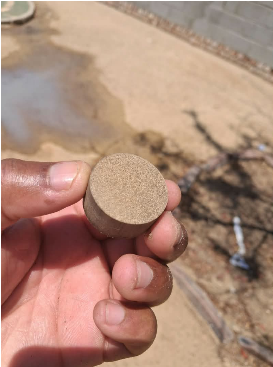
Image 3: Homogenised sample produced using the on-site lab facility at Uis, with the sample undergoing compression using the pellet press before being analysed, operated by trained Askari Metals geologists
