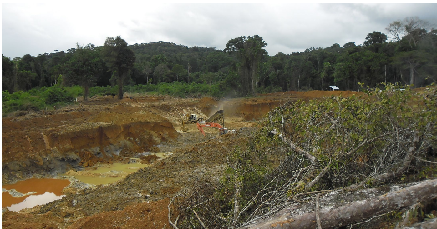
Figure 3 – Excavator-assisted workings on the Gonini Project with small-scale pump-and-slucie operation on the pit floor [circa 2020].
