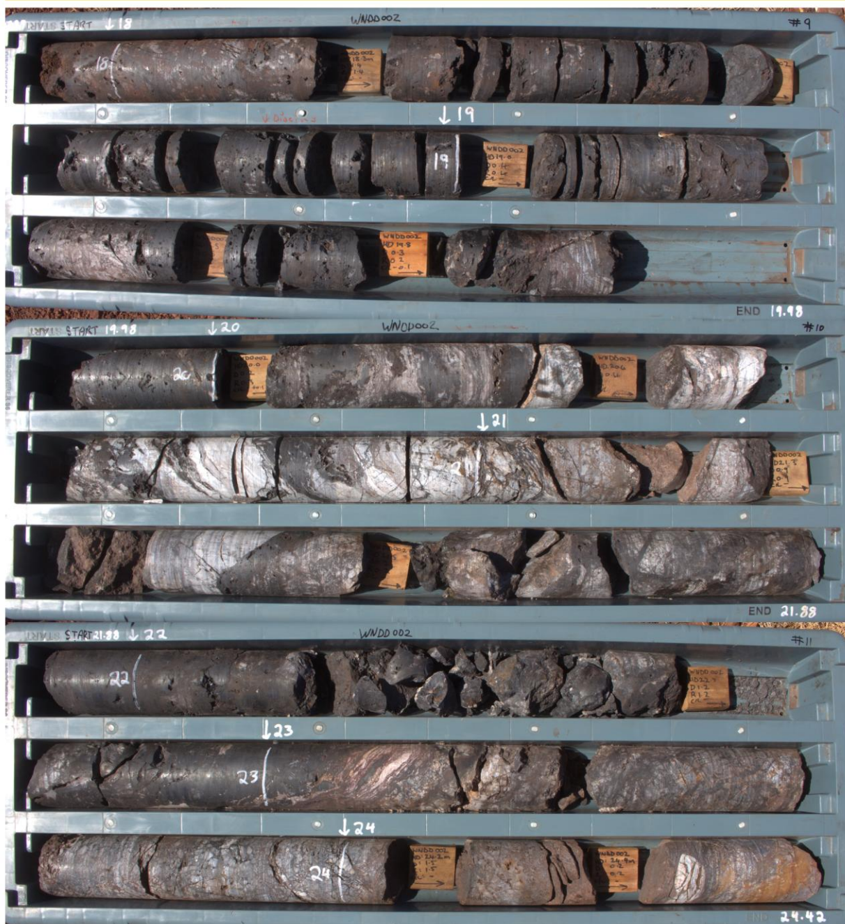
Figure 7, 8 & 9: WNDD002 trays 1 to 11 composite drill core photograph showing visual manganese (Visual observations only. Core photographs are not a proxy or substitute for laboratory analyses and provide no information on manganese grade, impurities or deleterious physical properties.)
