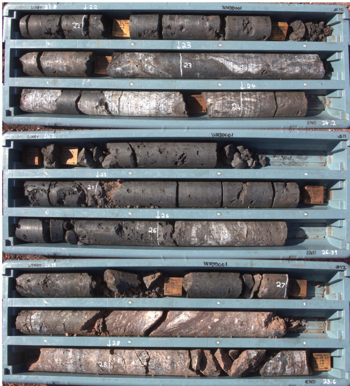
Figure 5 & 6: WNDD001 trays 6 to 12 composite drill core photograph showing visual manganese (Visual observations only. Core photographs are not a proxy or substitute for laboratory analyses and provide no information on manganese grade, impurities or deleterious physical properties.)
