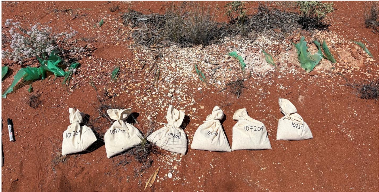
Figure 3: Samples from numbered remnant sample bags, historical RAB hole MMB0018 on Grid F.
