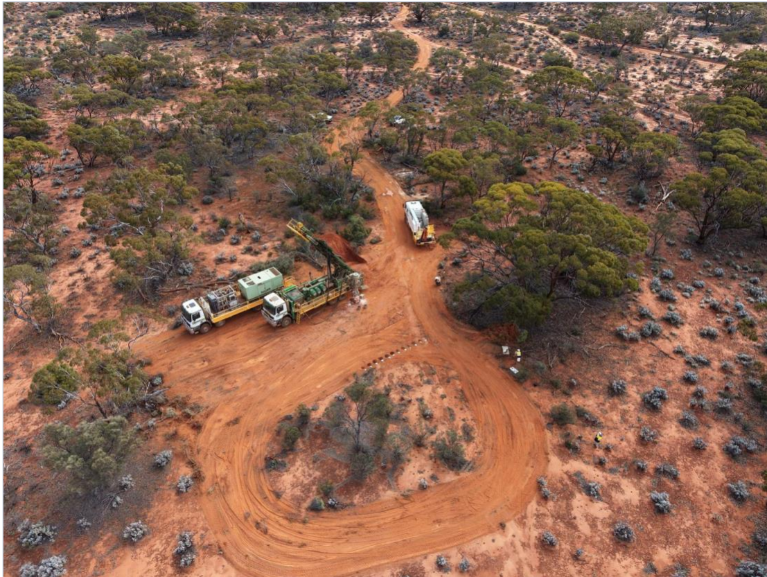
Figure 3 - First-phase RC drilling in progress at the Yindi Gold Project, central corridor (26YRC001).
