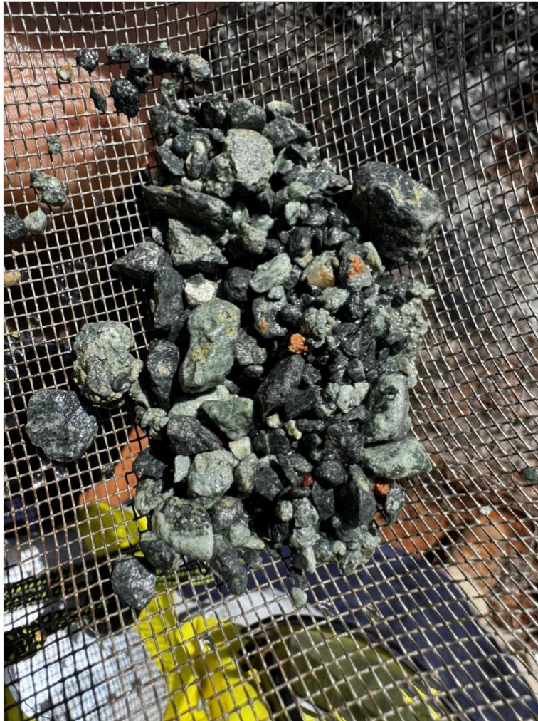
Figure 5 - RC chips from 26YRC003, 88–89m, showing chlorite-altered mafic rock with pale sericite–quartz alteration patches below the base of complete oxidation.
