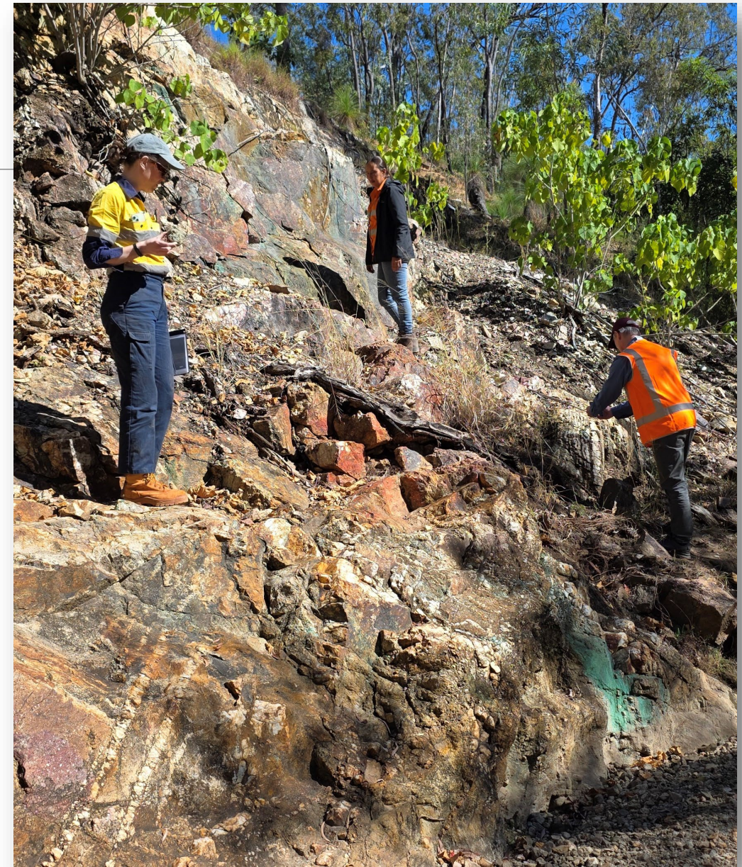
Quartz stockworks, sheeted veins and unidirectional solidification textures (UST) in outcrop in the centre of the Briggs deposit. Outcrop is above drill hole 25BRD0038, which intersected 386m @ 0.26% Cu from 7m, including 30m @ 0.90% Cu directly below this outcrop.
